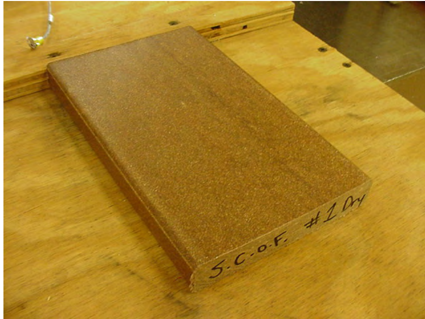
Photo No. 1 Test Specimen (Jatoba-colored Fiberon ® Tropics Decking)
